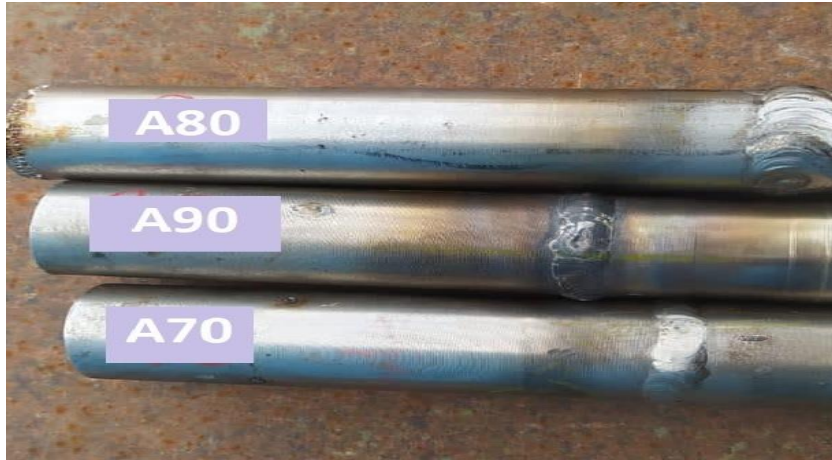
Figure (1) 316 Stainless steel welded specimens
