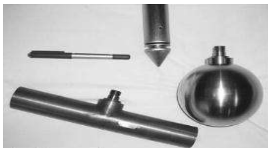
Fig (2) Cone ,T-bar & Ball shapes used in this study
